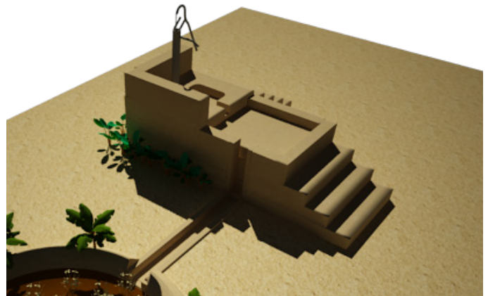
DRR-compliant elevated water pump accessible during floods.
