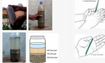
Soil should be checked with tests to ensure that the soil has clay content of 20%-40%. Methods for testing are Bottle Test and Coil Test.
