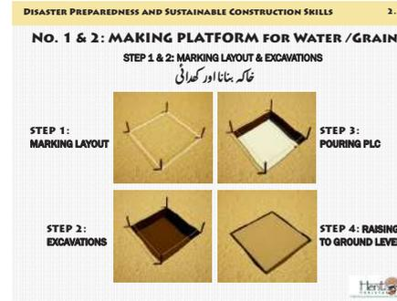
Mark layout 3'-6" x 3'-6"; dig 1'-6" after removal of 6" top soil. Place stakes on corners & pour 4" thick PLC. Raise wall in mud lime bricks.
