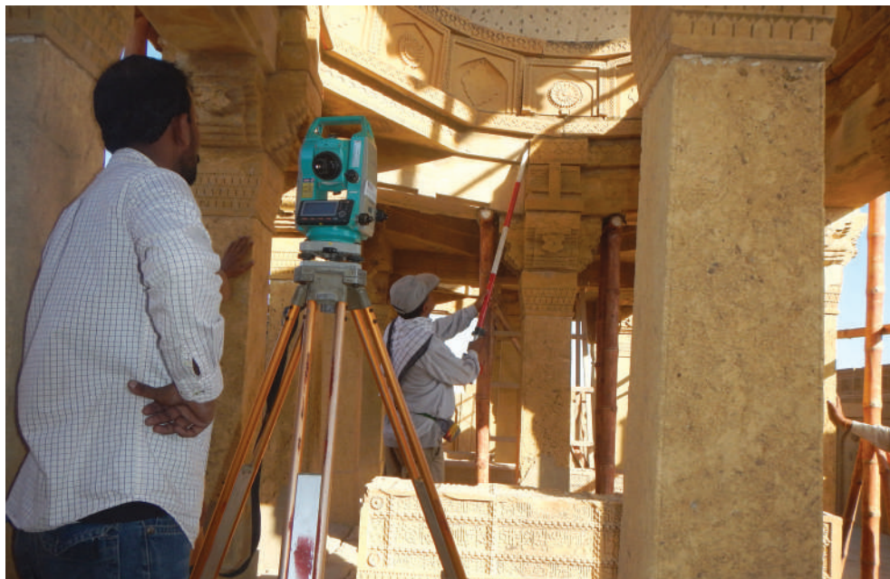
(Above). Survey drawing for road level and establishing the datum. (Right). Using instrumentation to determine movement.
