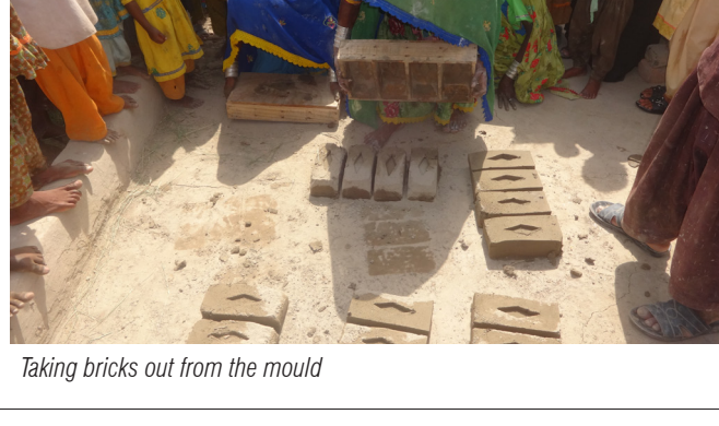
Taking bricks out from the mould
