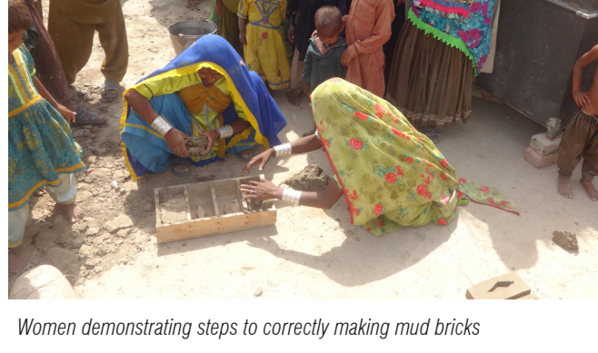
Women demonstrating steps to correctly making mud bricks
